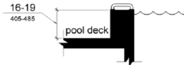
Figure 1009.4.2 Transfer Wall Height
